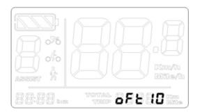
Display will sleep and cut off power after no operation on system for the setted time. Press M to save and skip to level amount setting.
