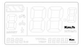
Then press (+) and (-) and no release, meanwhile press M eight times, to advanced setting.
