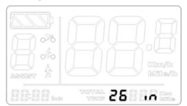
Press (+) or (-) to change the wheel size. Range from 8 to 32 inch. Press M to save and skip to sleep time interval setting.
