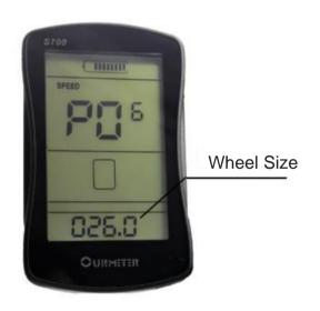
Switch to the P06 interface, press the "+" and "-" buttons to set the wheel diameter. If the wheel diameter is 26 inches, it is set to 26.0.
