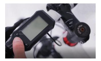
Install the display to the handlebar.
