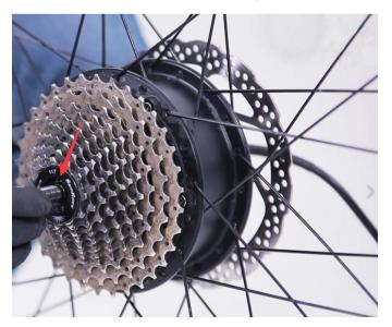
Install the cassette flywheel and lock the flywheel with the sensor cap. Note that it must be installed with the flywheel sensor cap of the system, otherwise there is no power output.
