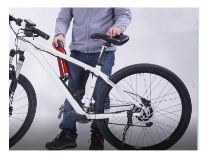
Install the battery on the battery holder.
