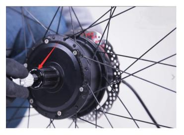
Remove the nuts and sensor cap from the cassette.
