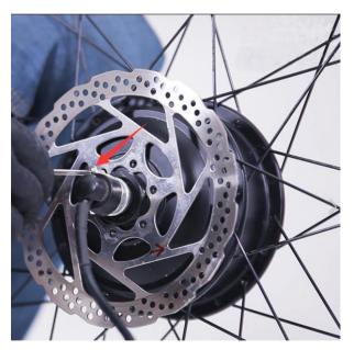
Install the disc brake using the 6 screws in previous step.
