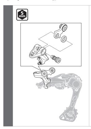
Remove the bracket axle.
