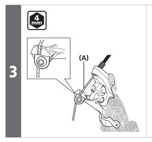
Reconnect the inner cable to the rear derailleur.
