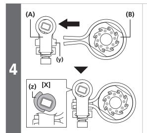
Set the chain stabilizer into the cam unit as shown in the illustration.
