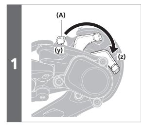
Make sure that the lever switch is in the OFF position.
