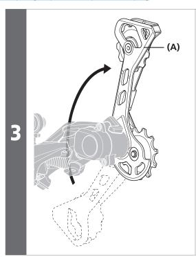
Turn the plate to loosen the plate tension spring as shown in the illustration.
