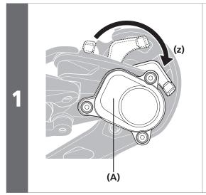
Make sure that the lever switch is in the OFF position.
