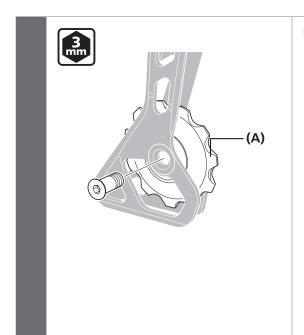
Replace the tension pulley.
