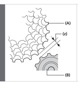
Set the rear derailleur on the largest sprocket, and with the wheel stopped, make sure that the clearance between the tip of the guide pulley and the tip of the largest sprocket is within the range (z).
