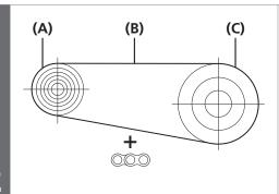
Mount the chain on to the largest sprocket and the largest chainring.
