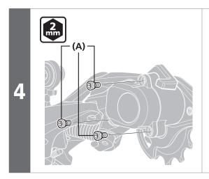
Remove the plate unit cover bolts.
