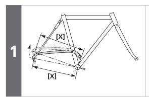
The length of dimension [X] will vary depending on the movement of the rear suspension.
