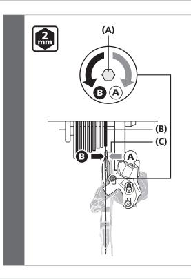
Turn the top adjustment screw to position the guide pulley over the outer line of the smallest sprocket when seen from the rear side.
