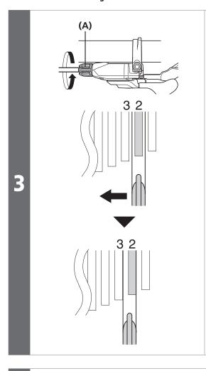
Loosen the cable adjustment barrel (counter-clockwise) until the chain touches the 3rd sprocket counting from the smallest sprocket and makes noise.
