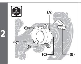
Using a 2mm hexagon wrench, remove the plate unit cover.
