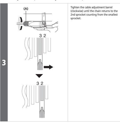
(A) Cable adjustment barrel
