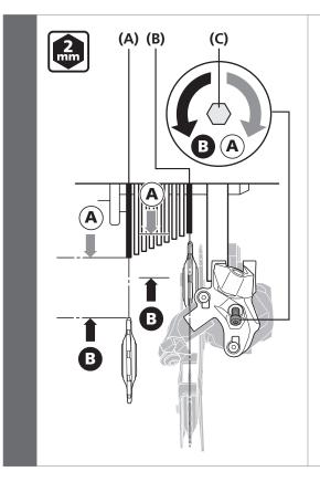
Mount the chain on the smallest chainring and the largest sprocket, and turn the crank arm to shift gears.
