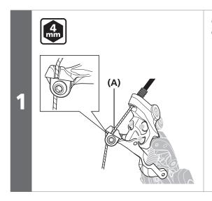
Connect the inner cable to the rear derailleur.
