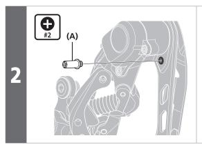
Remove the plate stopper pin with a screwdriver.
