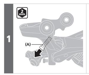
Loosen the end adjust bolt until it is in the position shown in the illustration.
