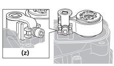
Align the holes in the cam unit and chain stabilizer with the projections on the plate unit and attach as in the illustration.
