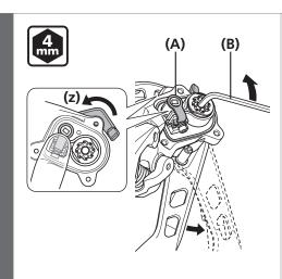
Check the friction torque.
