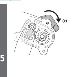
While pressing the friction unit with your finger, set the lever switch to the OFF position.
