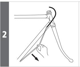
Remove the initial slack from the cable as shown in the illustration.
