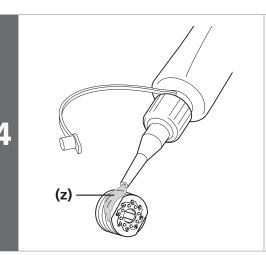
Apply grease to the clutch.
