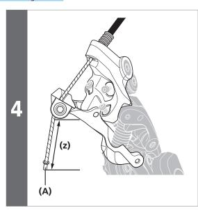
Set the inner cable so that the margin is approximately 30mm or less.
