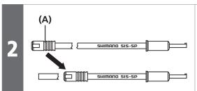
After cutting, attach the same sealed outer cap to the end.
