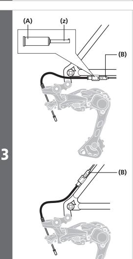
Install the sealed outer cap with tongue and the rubber shield onto the outer casing stopper of the frame.
