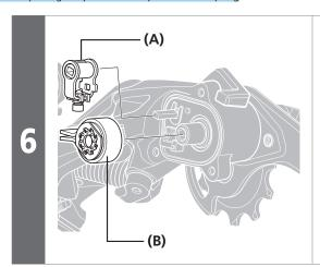
Remove the cam unit and the chain stabilizer.
