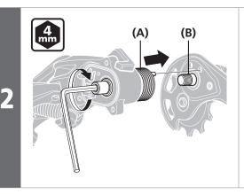
Insert the plate axle and insert the tip of the plate tension spring into the groove of the plate.
