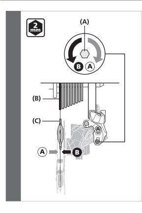
Turn the low adjustment screw to position the guide pulley directly underneath the largest sprocket.
